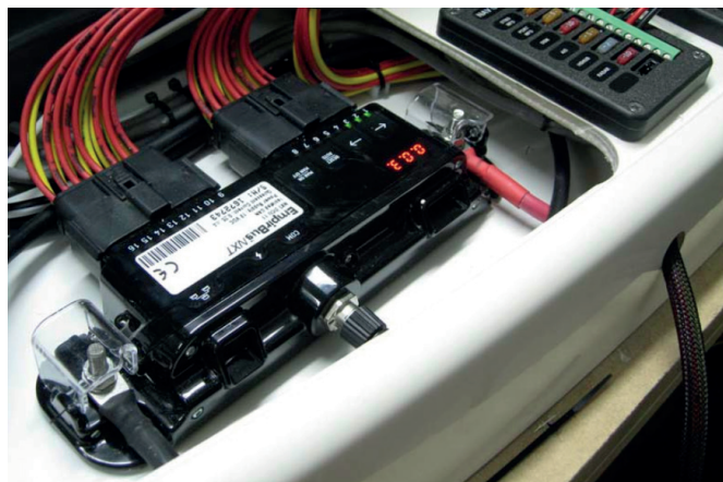
Master Control Unit installation showing connection of switchable devices
